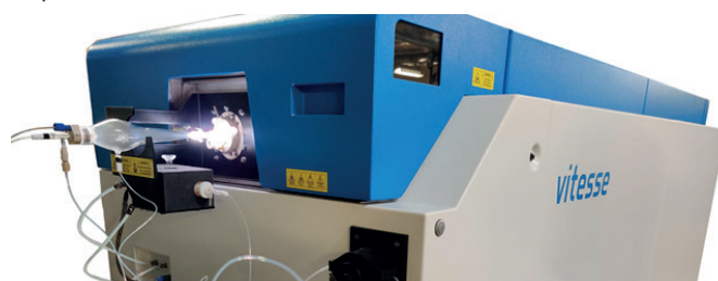
Figure 1: A typical setup for single cell analysis showing a specialized introduction system connected to the Vitesse.
