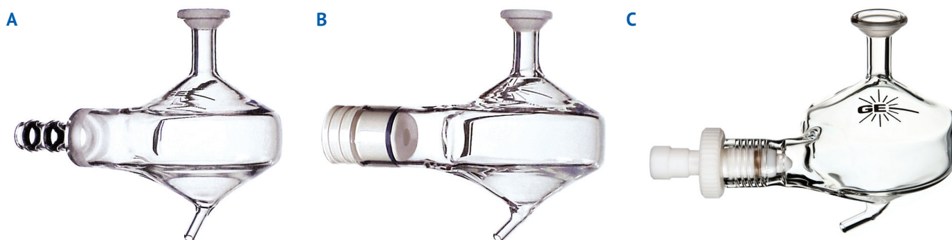
Figure 5: Progression of spray chamber-nebulizer interfaces; all glass with o-rings (A), plastic adaptor with o-rings (B), and Helix o-ring-free adaptor (C).
