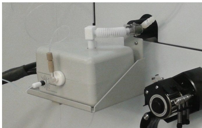
Figure 4: PCC Spray Chamber mounted on an Agilent 7700 ICP-MS
