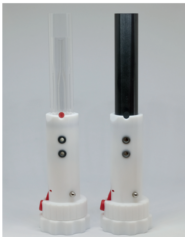
Figure 2. Conventional quartz torch and the new optional PLUS Torch for iCAP Qnova Series ICP-MS instruments
