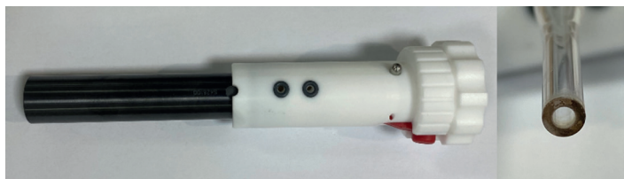
Figure 3. PLUS torch (left) and tip of the injector (right) after the repeated analysis of a mixed batch containing all sample types over 12 consecutive days
