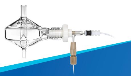
The Helix CT spray chamber with ConstantTorque<sup>™</sup> technology, provides a constant, reproducible, inert, gas-tight seal between the nebulizer and spray chamber. The Helix CT locking screw is equipped with a built-in torque control mechanism that allows for a consistent seal of the PTFE ferrule against the nebulizer,
