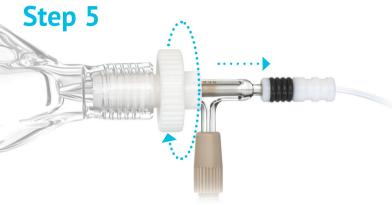
To remove the nebulizer, first loosen the fitting of the Helix by turning the Locking Screw counter-clockwise 1/2 turn, then slide the nebulizer straight out.
