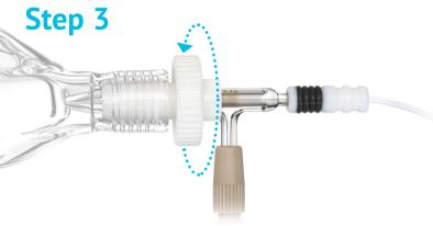
Tighten the nebulizer in place and seal the spray chamber by turning the knurled knob of the Helix CT further clockwise by hand until the ratchet mechanism clicks.
