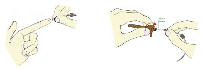
**Important Note:** Do not over tighten the thread cap, once you start to feel a bit of resistance with the thread cap, turn it another 1/4 of a turn and that should give you a reliable seal.
