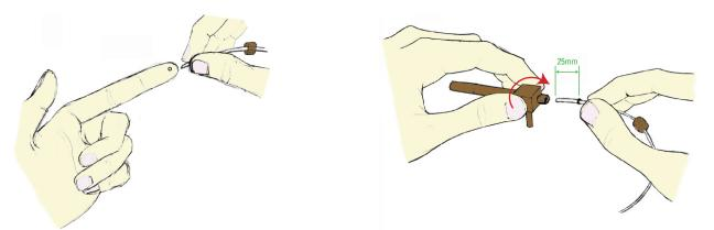
**Important Note:** Do not over tighten the thread cap, once you start to feel a bit of resistance with the thread cap, turn it another 1/4 of a turn and that should give you a reliable seal.
