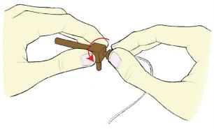
2. Cut a 45 degree angle on your NEW sample tube end by using a sharp blade, and insert it through the thread cap. Hold the end that you have just cut between your forefinger and your thumb. Make sure that the angle you have just cut is protruding no more than 2mm between your thumb and forefinger. Place the new o'ring onto your forefinger, and insert the sample tube through the o'ring so that the o'ring sits about 25mm away from the end that you have cut on an angle.
